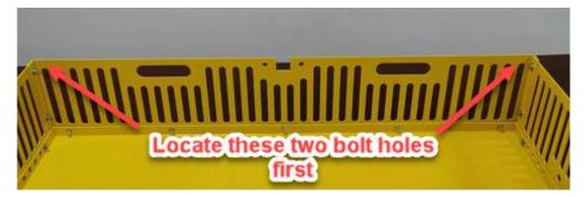
Identify the front brace (30mm x 30mm x 1085mm) and bolt in place using the M10\*20mm bolts supplied. Only place 1 washer on the nut side of the bolt. Finger-tighten bolts only.
